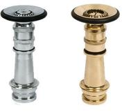
Triple purpose nozzles are combination nozzles, which give the option of hollow jet, protective spray or complete shut-off. Popular in industrial premises as they give the operator control over the discharge. The discharge can be varied by rotating the outer body, and the flow varies as the discharge changes from spray to jet.
